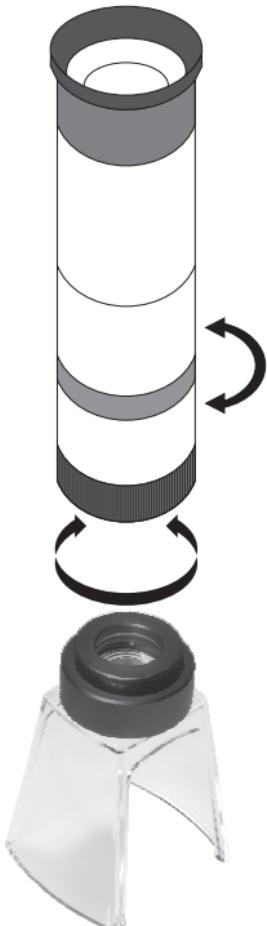
ular inwards and screw the standing magnifier onto the lens side of the hand monocular.
