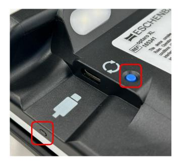
As long as the **LED connection indicator is orange** (or flashing), optaro® XL is in update mode and cannot be used as usual. If optaro® XL is switched off during the firmware update or the reset button is pressed, the update will be discontinued and the old firmware will remain in use.
